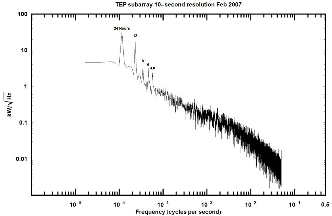
Figure 8. Power spectrum of TEP sub-array for 1 month at 10 second resolution. The sub-array low-pass filter behavior is shifted to higher frequencies relative to the full array (Figs. 6 and 7).
