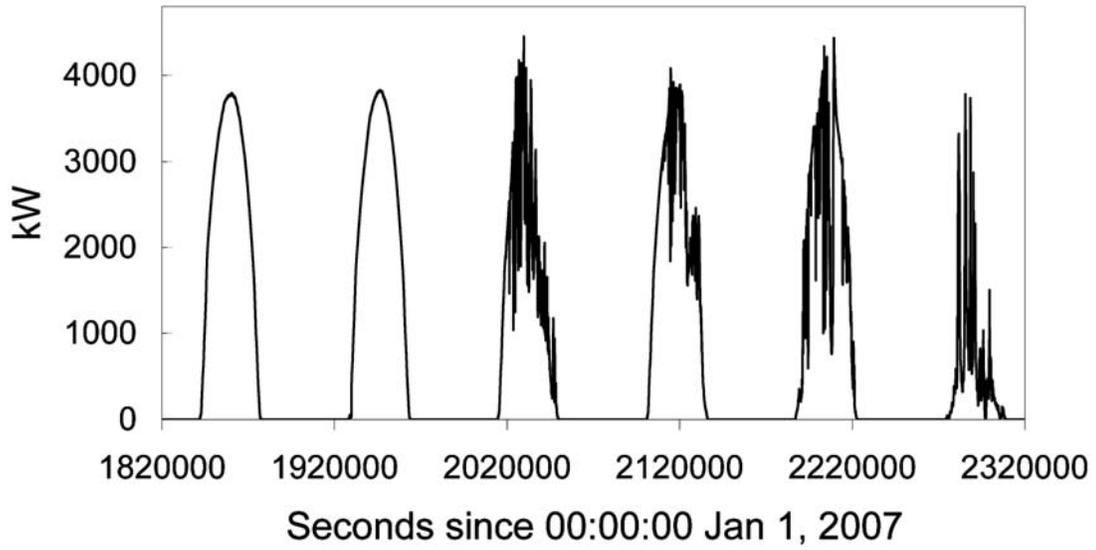
Figure 1. Real power output data from TEP over 6 days at 10 second sampling frequency.
