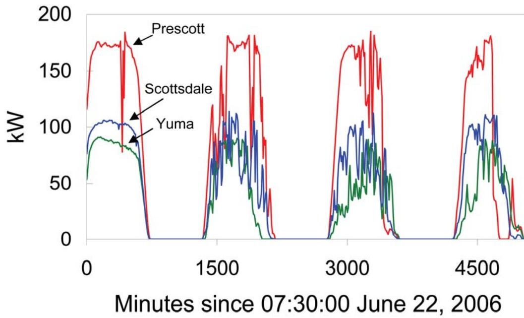
Figure 4. Real power output data from individual APS arrays over ~4 days at 10 minute resolution.
