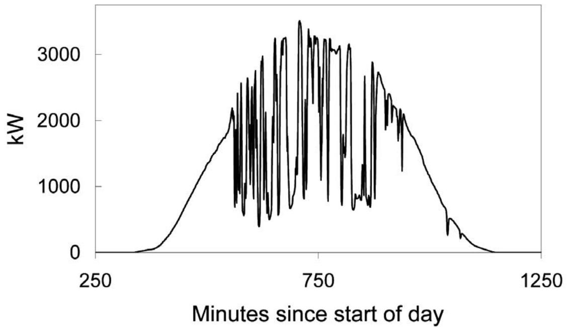
Figure 2. Real power output data from TEP over one full day in summer (June 3, 2004) at 1 minute sampling frequency.
