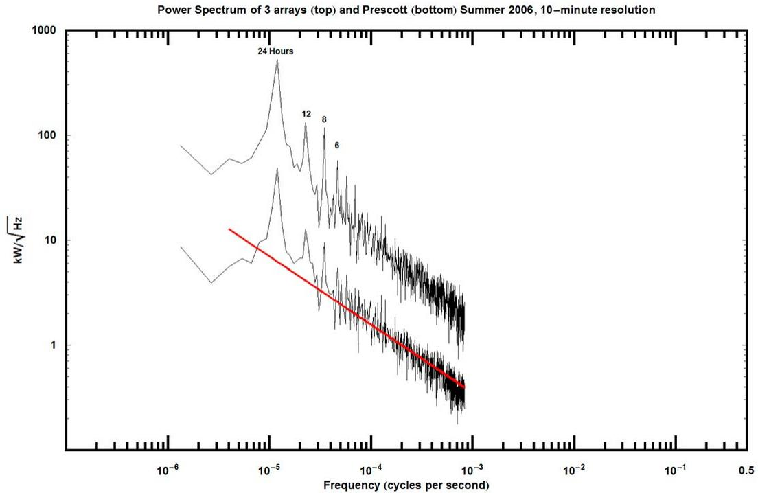
Figure 9. Power spectra of APS tracking PV arrays for 35 days at 10 minute resolution. Prescott site (lower spectrum) with overlaid  $f^{-1.3}$  spectrum and sum of all three APS sites (upper spectrum). The upper spectrum has been multiplied by 5 to offset the two spectra for clarity.
