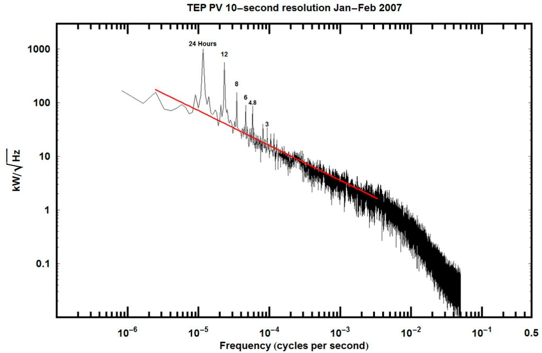
Figure 7. Power spectrum of TEP array over 2 months at 10 second sampling frequency with overlaid  $f^{-1.3}$  spectrum.
