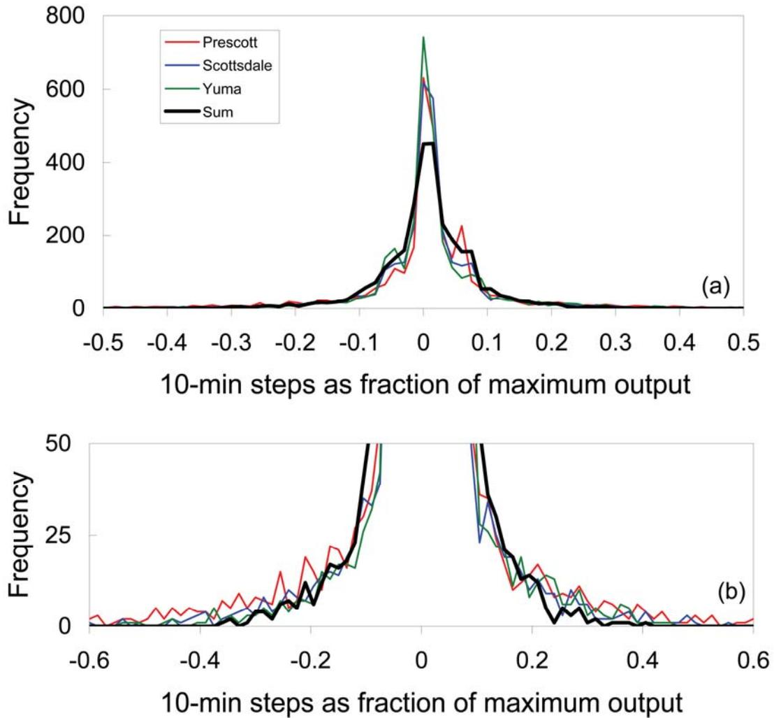
Figure 5. Change in fluctuation of power output from APS arrays with site diversity: (a) histogram of 10 minute steps (daylight only) and (b) detail of the tails of this distribution.
