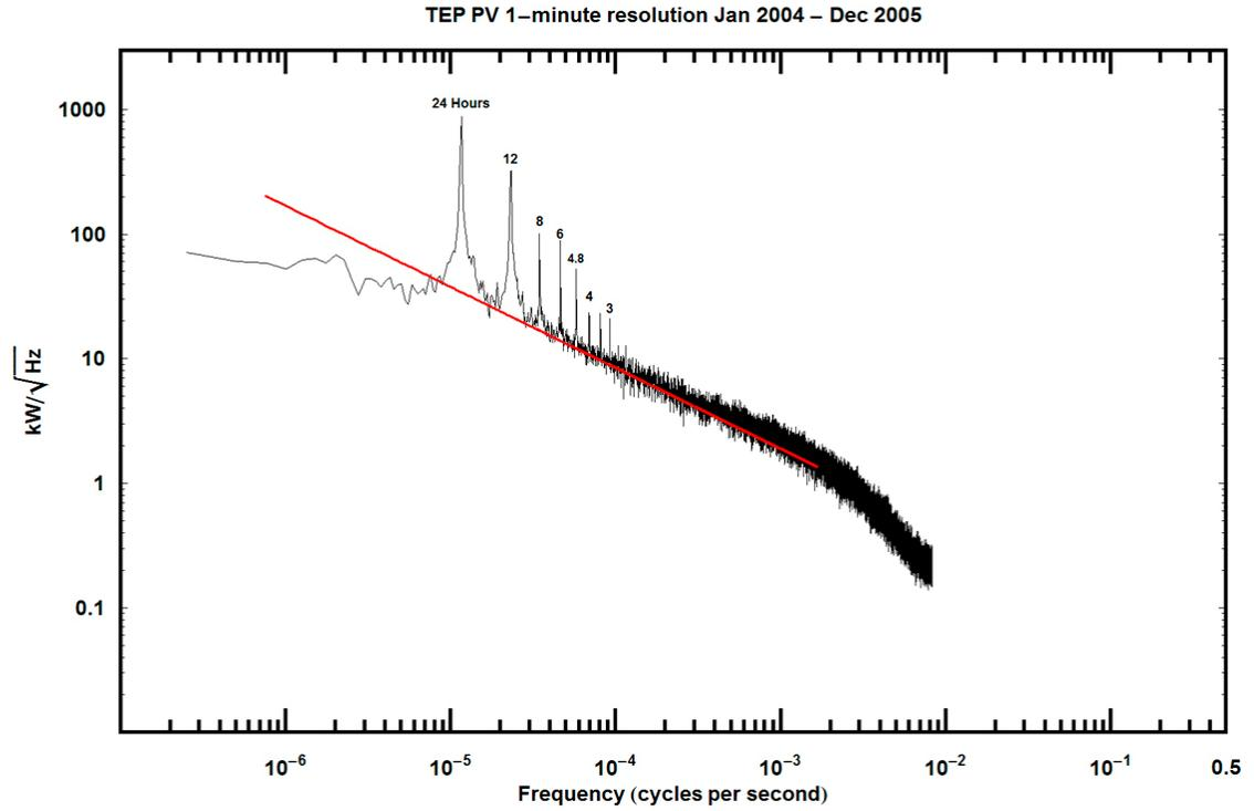
Figure 6. Power spectrum of TEP array over 2 years at 1 minute sampling frequency with overlaid  $f^{-1.3}$  spectrum.
