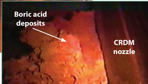
Figure 3b. Boric acid deposits accumulating near a CRDM nozzle (still photo of video taken during the 2000 refueling outage at DBNPS)
