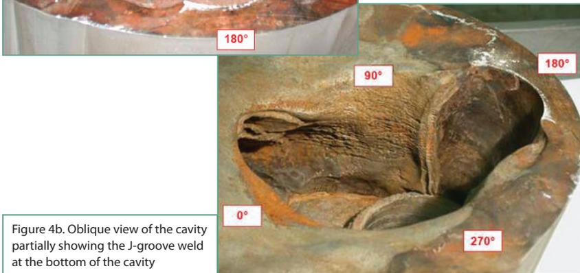
Figure 4b. Oblique view of the cavity partially showing the J-groove weld at the bottom of the cavity
