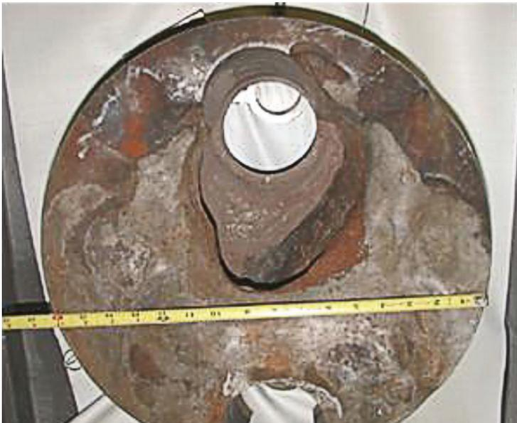
Figure 2. Region of the vessel head depicted by the model and photo of the cavity after it was removed from the vessel head
