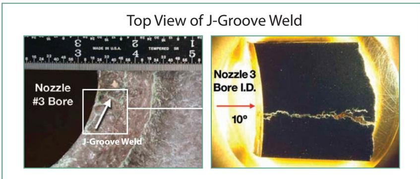
Figure 6. Top photo: Top view of the J-groove weld with an arrow pointing to a crack
