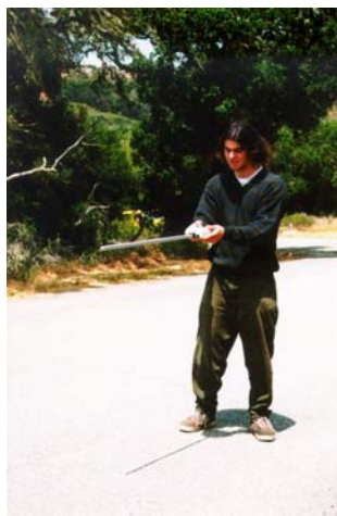
Figure 11. The AccuPAR sensor: for measuring leaf area index in the field.
