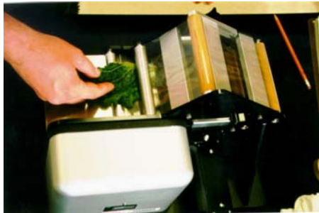
Figure 10. Measuring the area of lettuce leaves with a planimeter.
