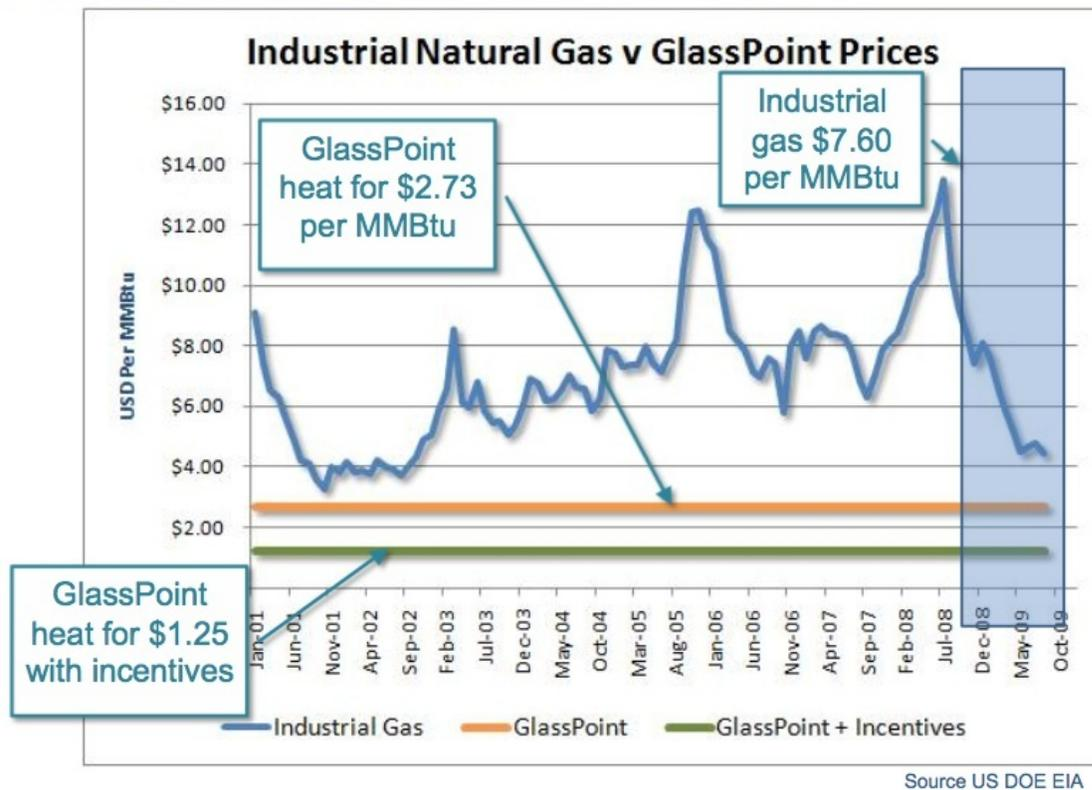
According to the material I was provided, the cost of heat is \$2.73 per MMBtu, using NREL's 30 year level cost of energy calculation. With incentives, the cost is quoted at \$1.25 per MM Btu, but I am not certain how the latter price is calculated. One incentive is a Federal tax credit of 30% available of installations begun in 2010. In California, there are also salable credits associated with California Cap and Trade laws. Since there are no carbon emissions, it avoids EPA regulation.
