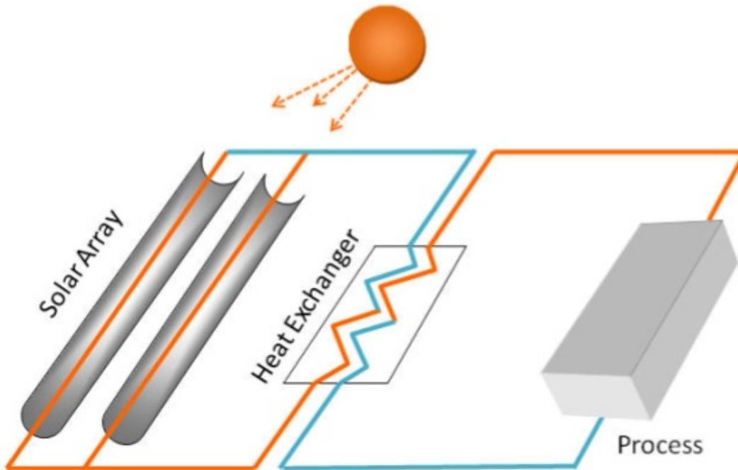
The above image indicates the GlassPoint's methodology uses solar concentrating mirrors which appear not to be movable. MacGregor indicated that nearly the entire ground surface is covered by the mirrors, since the mirrors are relatively cheap, and shadowing by other mirrors is not a concern. He also indicated that the mirrors incorporate some sort of self-cleaning mechanism.
